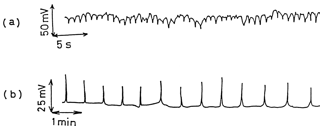
Fig. 2. Self-oscillation of electric potential in Millipore membrane impregnated with 2C_{18}N^+-PSS^- ( 0.63 \text{ mg/cm}^2 ). a: 35^\circ\text{C} , b: 50^\circ\text{C}
